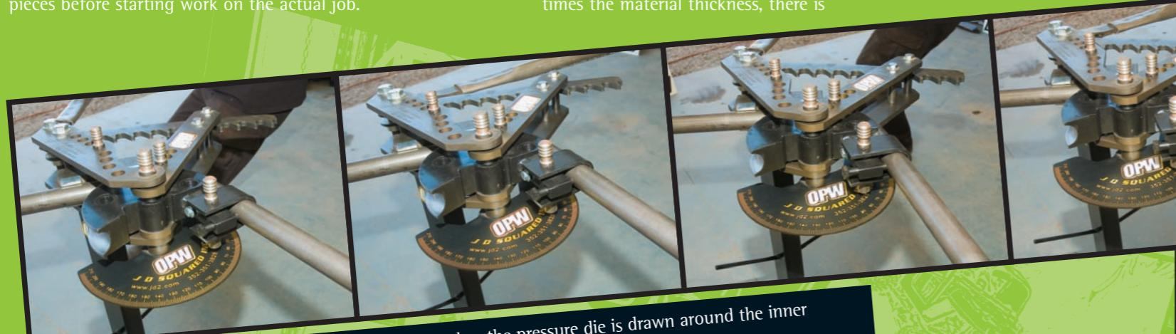
Above: The U-clamp holds the tube in place and as the pressure die is drawn around the inner forming die, bending the tube to the desired angle.
